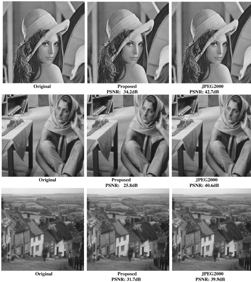
Fig. 19. Reconstructed images: compression factor 4:1, 64 \times 64 tile, 4-levels 5-3 DWT.
