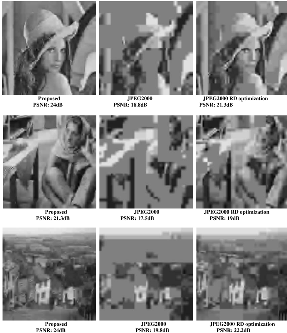
Fig. 18. Reconstructed images: compression factor 160:1, 64 \times 64 tile, 4-levels 5-3 DWT.
